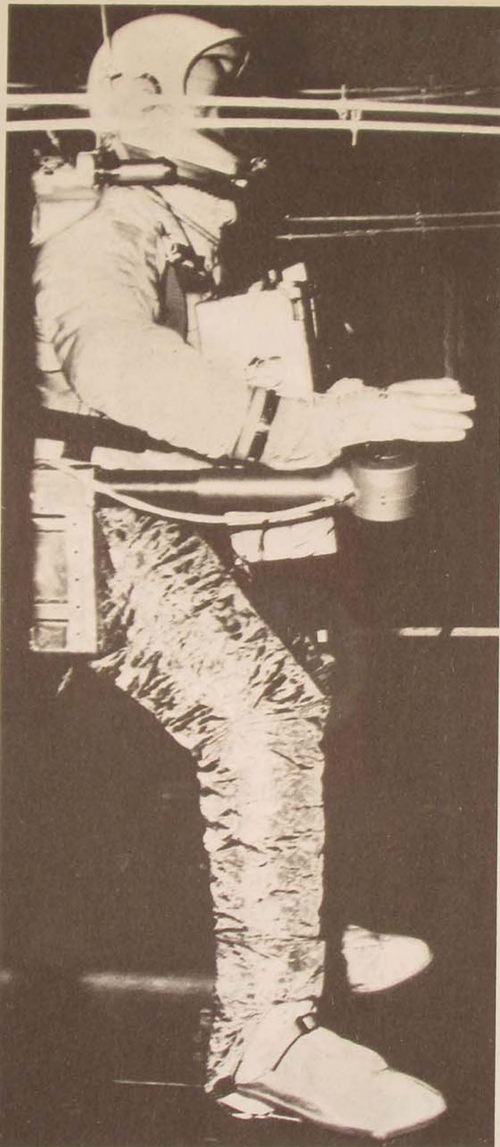
The astronaut's metallic coverall is fabricated from Chromel R, developed by the Air Force Materials Laboratory. It is worn during extravehicular activity and protects him from the 1200°F gas plumes that shoot from the jet thrusters of the Astronaut Maneuvering Unit.
