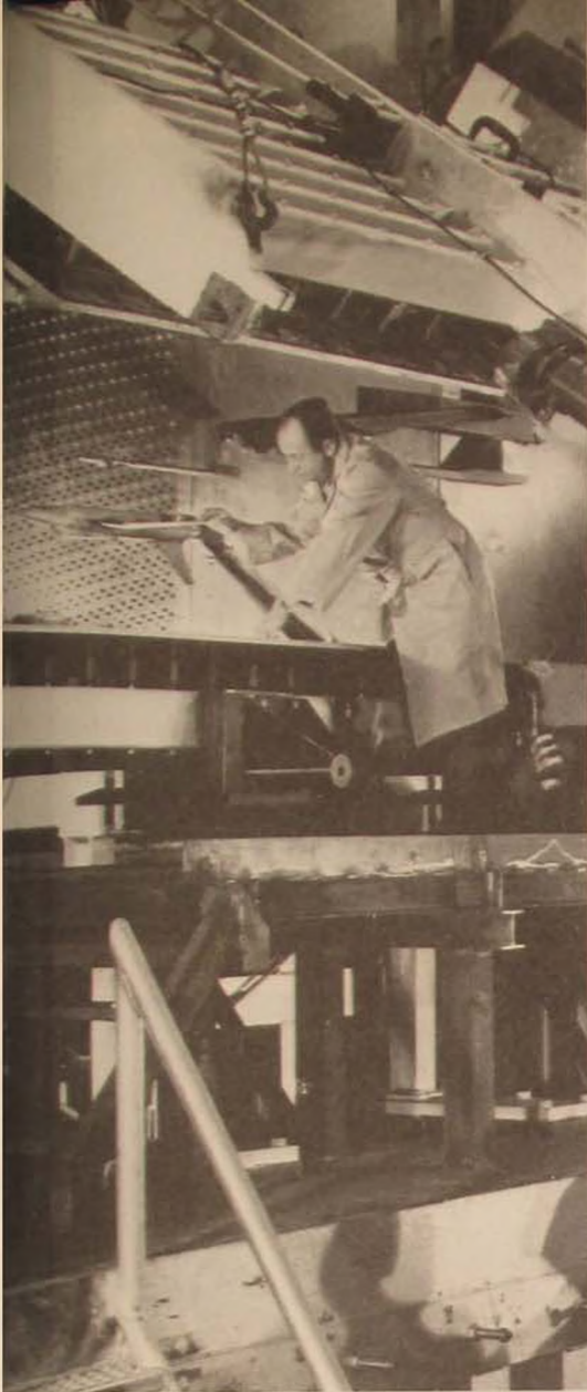
The lowered cryogenic walls of the Mark I aerospace environmental chamber use liquid nitrogen and gaseous helium to attain a vacuum of 10^{-8} Torr (approximately 300 miles altitude) and temperature of 72°K (-340°F). . . . The transonic wind tunnel is used primarily for stores separation tests. Models are mounted upside down to aid in equipment-handling problems. . . . Velocity measurements in high-speed, high-temperature gas flows are made with a pulsed ruby laser and image converter camera.
